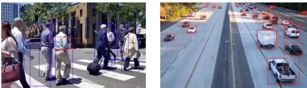
Figure 2: Screenshots from video of Centroid performing object detection on eight 1080p30 streams running at a throughput of 500 megapixels per second (MP/s).
